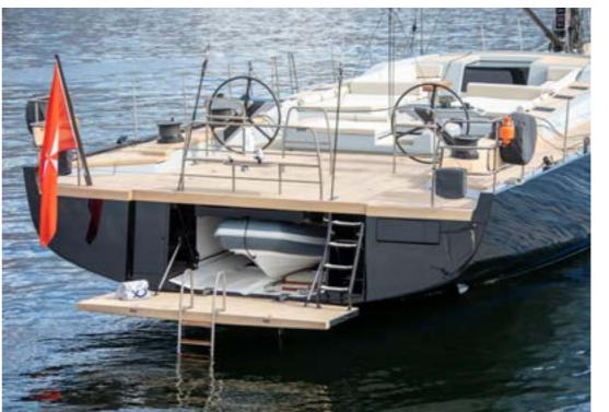
FAST AND FUN: SØRVIND is built with a full carbon hull, deck and bulkheads. Weight control has been a high priority with major savings thanks to the titanium deck hardware and FlexiTeek decking. This results in a high performance and reliable yacht that can sail in a wider range of wind conditions, with a reduced dependency on the engine.
